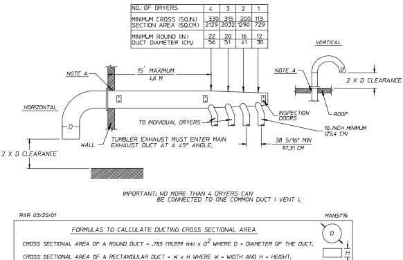
NOTE A: OPENING MUST BE 2-INCHES (508 CM) LARGER THAN THE DUCT (ALL THE WAY AROUND) THE DUCT MUST BE CENTERED WITHIN THIS OPENING.
